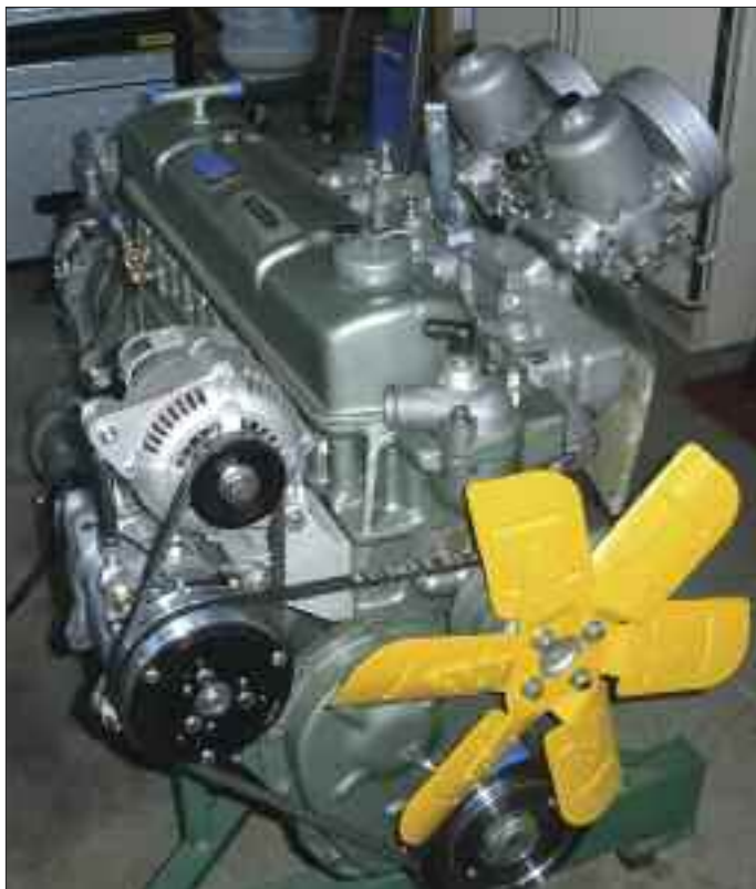
Interesting setup of an alternator and air conditioning compressor fitted to a six-cylinder engine.
