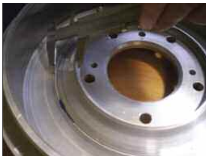
Measuring the new drums.
